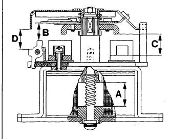
DIMENSION C = GAP BETWEEN BUSBAR AND CONTACT BRACKET
